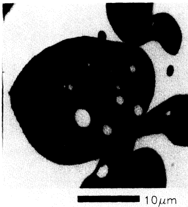
Figure 2 Micrograph of 0.5 \mu\text{m} thick section of poly(styrene- r -acrylonitrile)/polypropylene blend acquired at a photon energy of 285.5 eV. Styrene is strongly absorbing at this energy and the phase containing it appears dark, while polypropylene is virtually transparent. Black and white levels of the micrograph are from zero to incident intensity, i.e. contrast is not digitally or chemically enhanced. This micrograph was one of the very first to demonstrate the chemical capabilities of the X1-STXM
